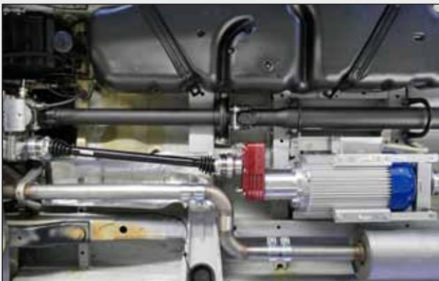
The generator needed to generate electricity is driven via the vehicle engine and a factory installed auxiliary drive which should be considered when ordering the vehicle.
